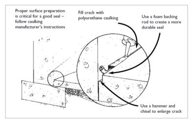
All penetrations of a floor-on-ground by pipes or other objects shall be sealed against soil gas leakage.
