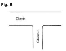
c) The angle of the intersection must not be less than seventy-five degrees (75°) and right-angled intersections are the preferred option. Alignment must be maintained over a minimum distance of thirty (30) metres;
