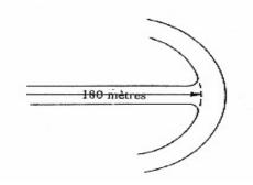
e) No intersection shall be located on the concave (exterior) edge of a curve with radius less than one hundred twenty (120) metres;
